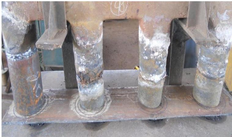
Stub pins as per marking in testing plate. If any stub pin crosses the outer ring marked (160mm) in testing plate mark it for pin cutting. Check the height of stub pin to be cut with the help of measuring tape. Write the height of round bar which is to be cut above bracket.
